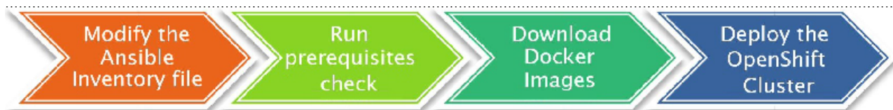
Figure 9 Process for a single-node installation of OpenShift OKD
